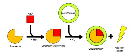
ATP, in the presence of a luciferin/luciferase complex with a catalyst, releases energy in the form of light. By measuring the amount of light emitted using a luminometer, we deduce the quantity of ATP in picogram per cm<sup>2</sup>. The total flora, expressed in equivalent bacteria per cm<sup>2</sup>, is calculated from the following:
