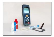
Thaw a dropper bottle of each reagent (DENDRIDIAG® BF, EXTRACTANT and STANDARD 1000). Bring them to room temperature (above 18°C).
