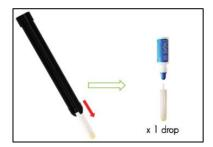
Immediately, get the tube holder with the test tube out of the luminometer.
