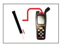
Fix the tube to the tube holder.
