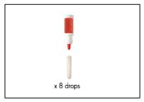
Make sure the reagent **EXTRACTANT** is close to room temperature (> 18°C) and put 8 drops of **EXTRACTANT** in the middle of the test tube.
