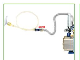
2. Connect the assembly on the vacuum pump. Filter at the maximum flowrate for 10 minutes (volume filtered = 70 liters).
