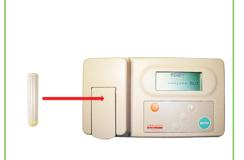
8. Place the tube in the luminometer. Press ENTER to start the analysis. Write down the result R2 (in RLU).
