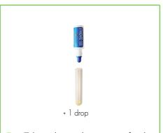
7. Take the tube out of the luminometer and add one drop of **STANDARD 1000**.
