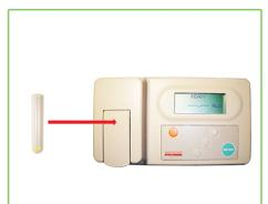
6. Place the tube in the luminometer. Press ENTER to start the analysis. Write down the result R1 (in RLU).
