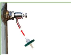
2. After flushing the sampling point, connect the filter-connector to the PEMS II valve. Filter one liter of water (measure the volume filtered by filling a waste container).
