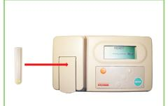
8. Open the luminometer and place the test tube inside the measurement chamber. Start the analysis by pressing the ENTER button. Write down the R2 result (in RLU).
