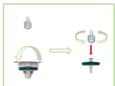
1. Open the cap of the filter packaging (do not discard the plastic packaging). Connect a luer-lock connector to the filter being careful not to touch the components' tips.
