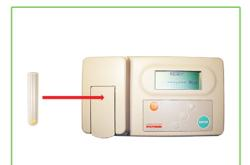
6. Open the luminometer and place the test tube inside the measurement chamber. Start the analysis by pressing the ENTER button. Write down the R1 result (in RLU).
