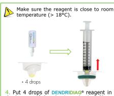
4. Put 4 drops of DENDRIDIAG® reagent in the bottom of the plastic packaging. Place the filter tip in the plastic packaging. Suck up all the reagent and maintain the depression in the syringe.
