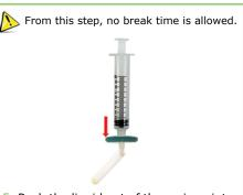
5. Push the liquid out of the syringe into a test tube until a white foam comes out. Stop the pressure as soon as the foam comes out to avoid creating a « stopper » in the upper part.
