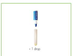
7. Immediately after the first measurement, get the test tube out of the luminometer and add one drop of **STANDARD 1000** in the middle of the test tube.
