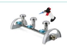
1. Sterilize each filter holder of the manifold with flame and alcohol. Let them cool down a few minutes before placing the membranes on top.
