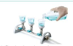
$4.\,$  Open the valves and turn on the vacuum pump to start filtration of the samples. Avoid drying the membranes for too long.
