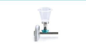
3. Place the sterile funnels (plastic or stainless steel) on the filter holders, above the membranes. The filters should not be fold. Fill the funnels with the water samples.
