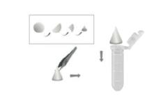
5. When filtration is over, close all the valves and remove the funnels. Fold the membranes as shown above and place each of them in a microtube containing TGBE buffer. The tip of the cone should point upwards.
