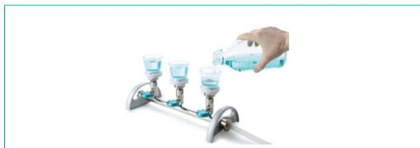
3. Place the sterile funnels (plastic or stainless steel) on the filter holders. Pour the sample containing the Binding Buffer into the funnels.
