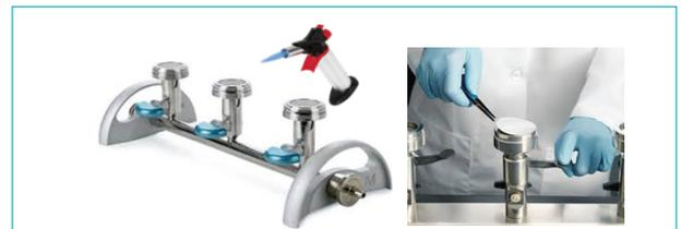
2. Sterilize each filter holder of the manifold with flame and alcohol. Let them cool down a few minutes before placing the membranes on top.
