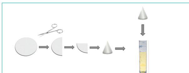
5. When filtration is over, close the valves. Cut the membranes in 8 parts using steril scissors. Place them in the tube containing 5 ml of Elution Buffer.
