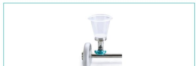
4. Open the valves and start the filtration. To ensure an optimal retention, apply a vacuum of 0.6 to 0.8bar.
