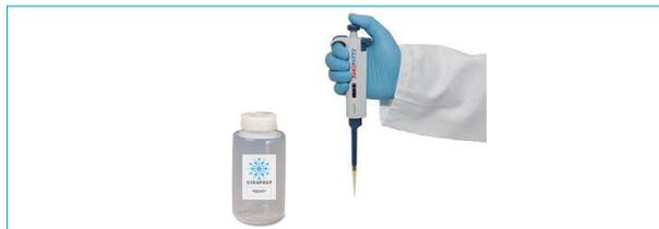
1. Add the Binding Buffer 50X in the sample to be analysed respecting the following proportions: 2 ml of Binding Buffer for 100 ml of water sample.
